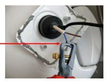
9. Thread the new pump cable through the plastic bracket.
