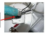
14. Re-connect the flushing tube and vacuum breaker and carefully replace the tube to the pump in the clips.
