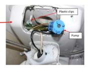
5. Pump with hoses disconnected
