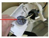
7. Cut the old pump cable as high as possible (to keep joints out of water)
