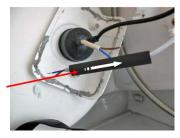
11. Push the bared wires into the connectors (blue to blue and brown to brown) and crimp with a crimping tool. Temporarily restore the 12V supply and try the pump before continuing. If the pump fails to work re-check the connections.
