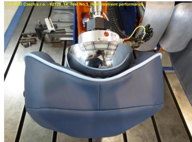
e) Head restraint energy dissipation test – front, 90°
