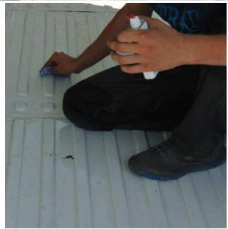
Clean vehicle bodywork before installing the floor. For this purpose use Betaclean (cleaner) to degrease the vehicle's floor and the underside of the composite floor.
