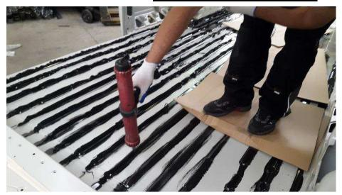
Apply Betamate on the vehicle floor. Primer should be dry.
